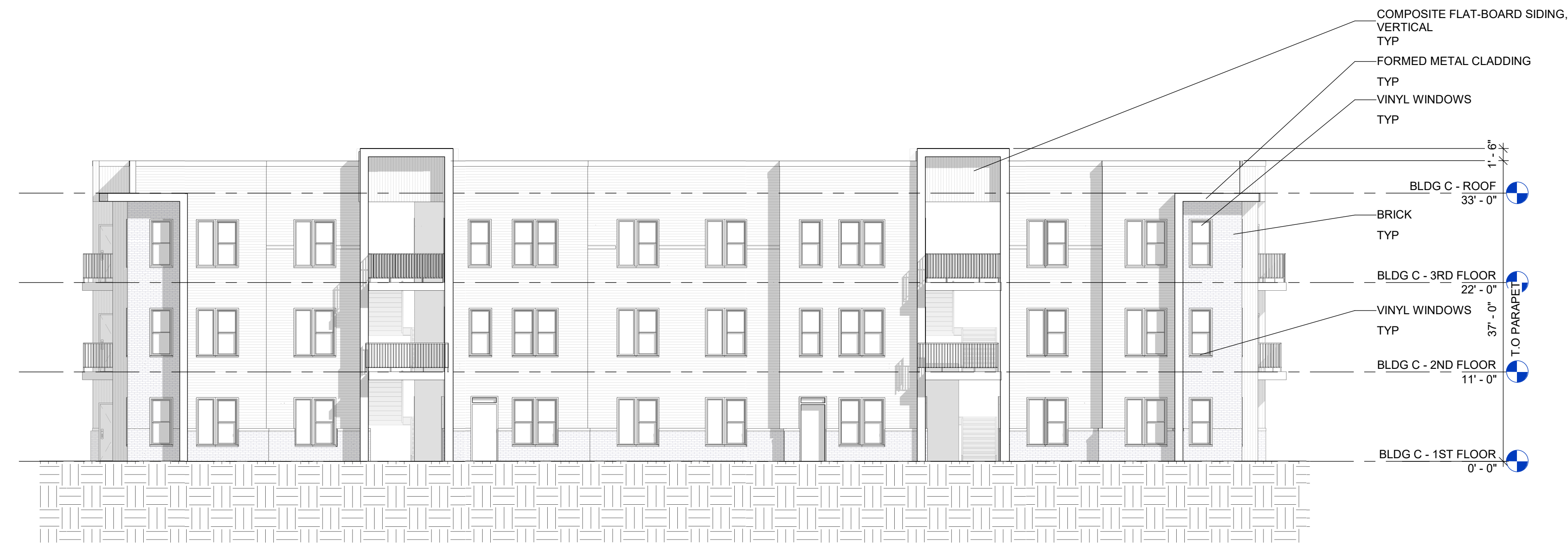
3 ELEVATION - BLDG B AND C - WEST 3/32" = 1'-0"
