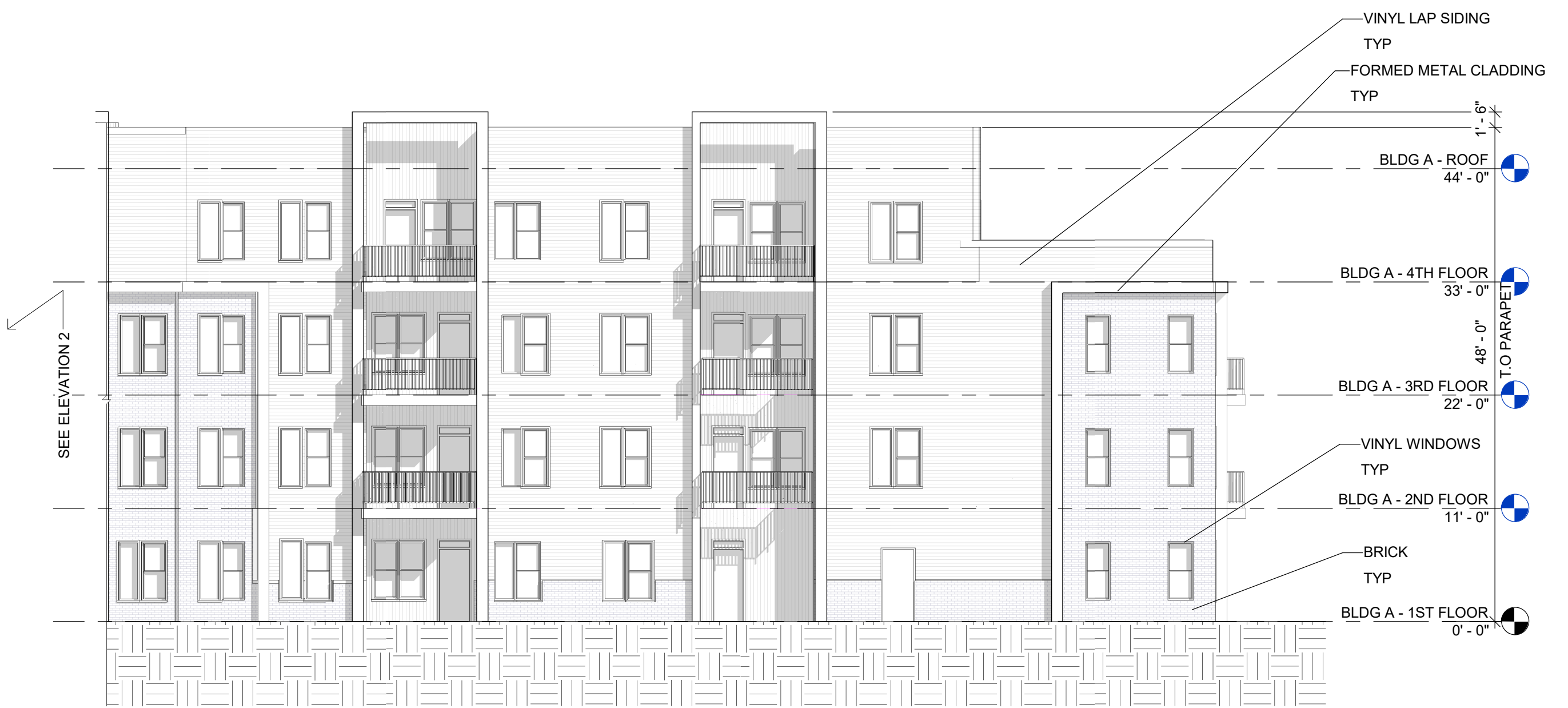
3 ELEVATION - BLDG A - SOUTHEAST 3/32" = 1'-0"
